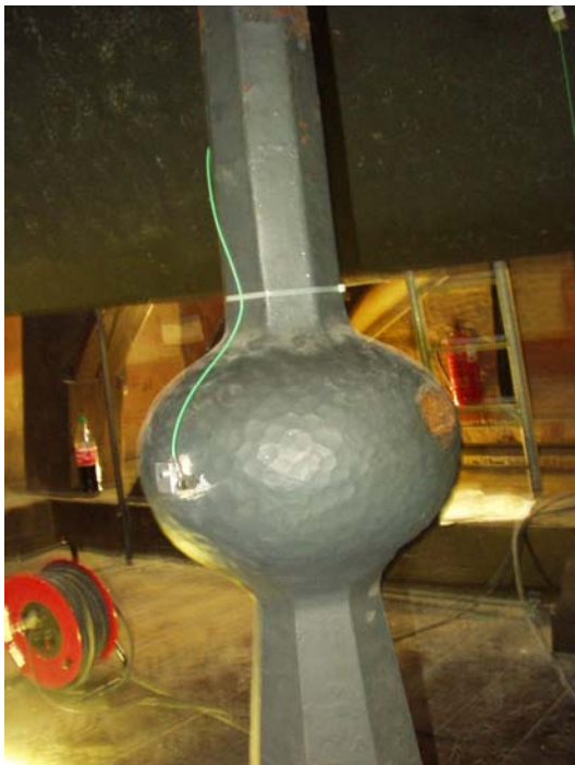
Fig. 4c: Accelerometer on a clapper
