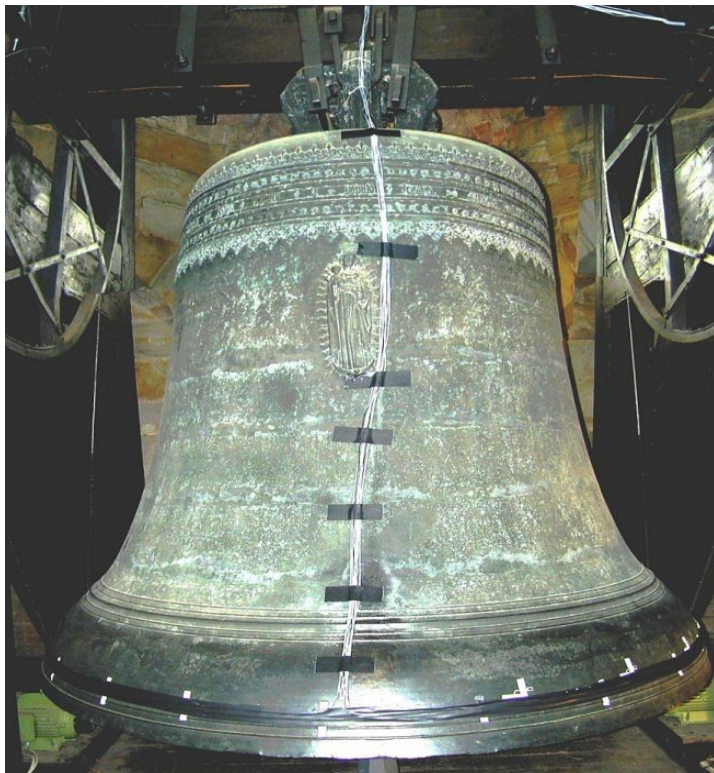
Fig. 1: Gloriosa with strain gages, Erfurt, casted in 1497,
